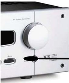
4. Self-adhesive “Flashers” affix to the Infrared sensors on the front panels of your components. The Flashers relay commands to components out-of-sight of the MRF-350's Front Blaster. The flashers plug in to the MRF-350's rear flasher line outputs via their 10 foot cables. Uniquely, the MRF-350 can also connect to components with rear panel IR Inputs via its adjustable IR Line Outputs.
