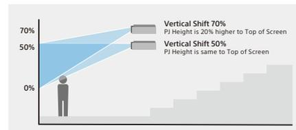
The projector has variety of lens options and wide lens shift capability for flexible installation, virtually anywhere.
